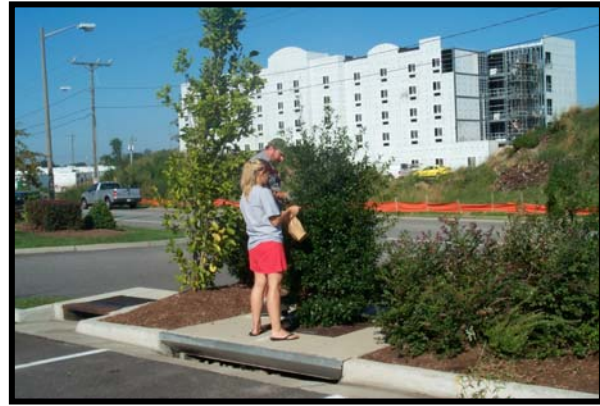
Figure 2 (left) – Hollies planted in Filterra ® units installed in a parking lot with replicate landscape holly in background. Figure 3 (right) – Collection of leaves from a holly for N and P analysis.
