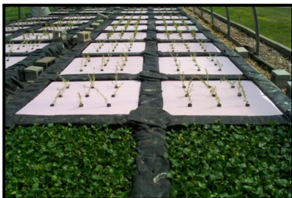
Figure 1 – The modified hydroponic system used to evaluate woody shrub accumulation of N and P. (In the foreground are the water hyacinths used to develop the protocol.)
